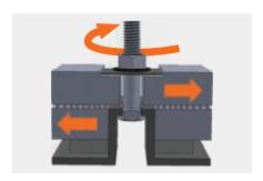
Standard pre-loaded fasteners can loosen as a result of relative motion between surfaces due to vibration. The J-Washer's knurled surface locks the nut when torque is applied so that no loosening occurs. The locking design has been verified by the industry standard Junker test, which simulates the transverse forces that loosen the assembly.
