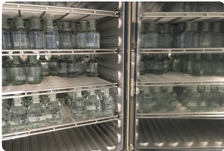
Biochemical Oxygen Demand (BOD) bottles in the incubator for use in the OECD 301D methodology.
