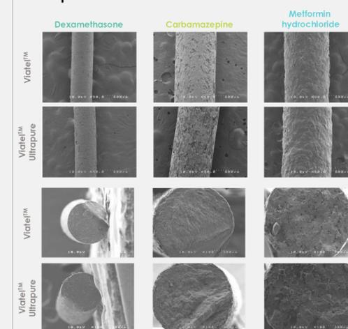
Implants' surficial and internal structures were characterized by SEM. All implants exhibited a rough, irregular surface. At the same processing temperature, Viatel™ ultrapure PLGAs led to a slightly worse surficial and interior structure than Viatel™ PLGAs did regardless the molecular weight difference, due to their lower contents of residual monomer (low plasticity).
