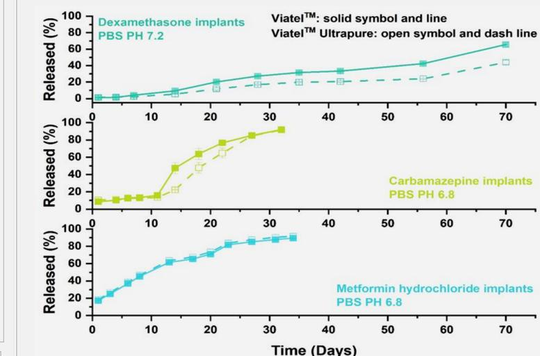
The implants with Viatel™ PLGA exhibited less burst release than implants with Viatel™ ultrapure PLGA, however, their onset and progress of the major release phase were shorter and faster than the Viatel™ ultrapure based implants, owing to the residual monomer catalyzed PLGA hydrolysis. In addition, the drug release profiles were also influenced by other factors, such as polymer-drug interaction and drug solubilities.
