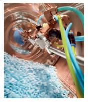
▲ on the cover commercial tablet coating process using Ashland aquarius" genesis tablet coating solution
