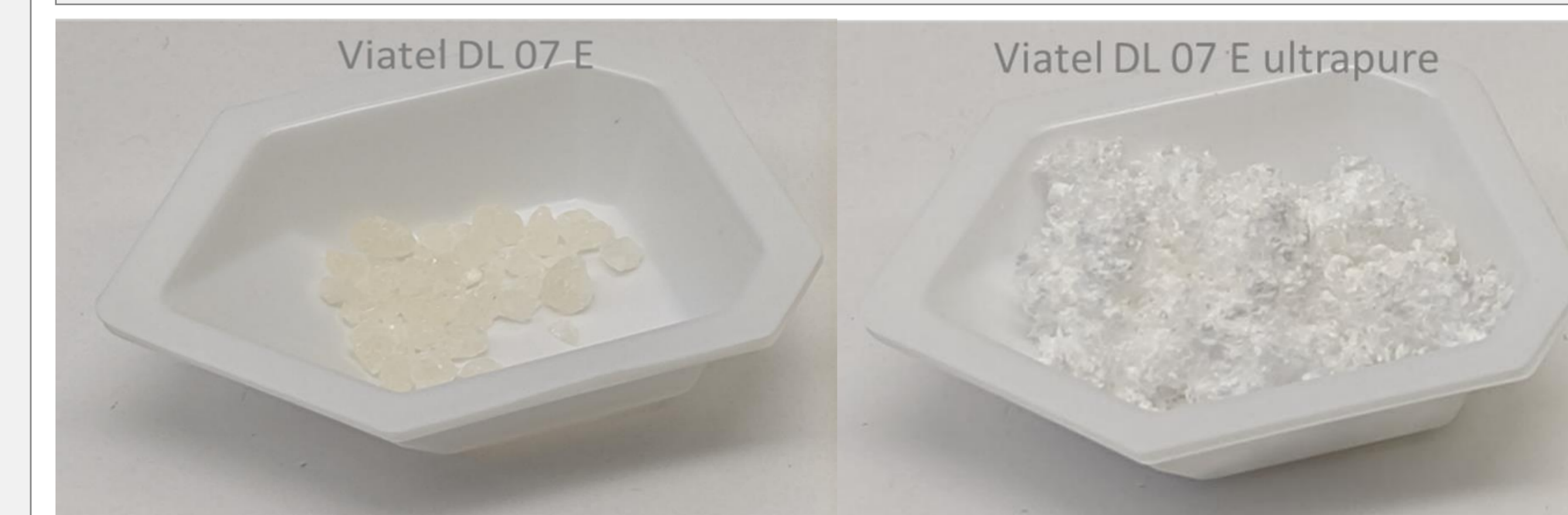
Image 1: Comparison of Viatel DL 07 E polymer (left) and Viatel DL 07 E Ultrapure polymer (right)
