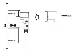
Fold in Dog Ears and slide Housing into wall.
