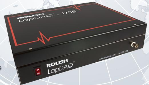
The size of a laptop computer, the Roush LapDAQ™-USB enclosure is an ideal, portable, ruggedized enclosure for your 5B signal-conditioning modules.
