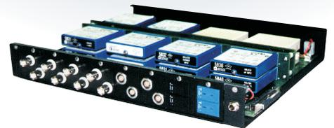
Inside this compact package is room for up to 16 5B signal-conditioning modules. A highly adaptable power supply is also built into the Roush LapDAQ™ enclosure.
