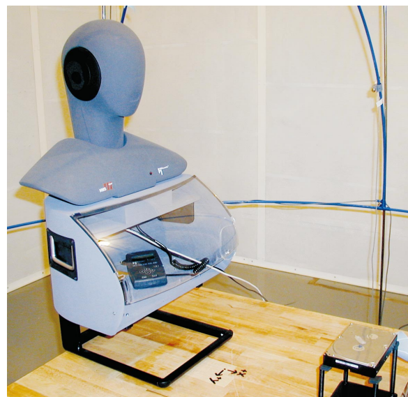
Figure 1 — Typical Binaural Head Recording Setup for an Operating Hard Drive
