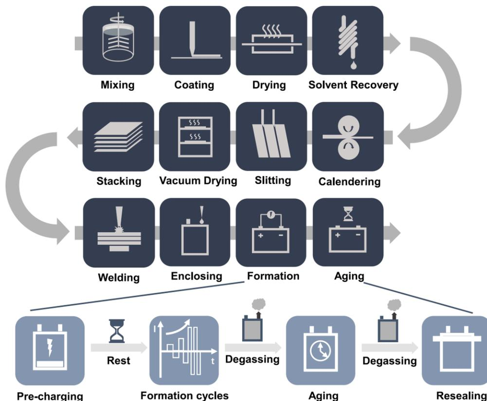
**Figure 43: Schematic of lithium-ion battery manufacturing processes [150]**
