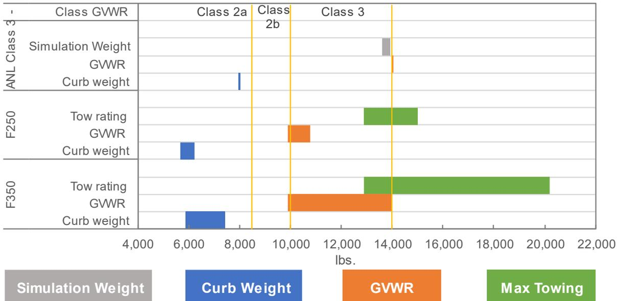
**Figure 14: Variation of the curb weight, GVWR, and maximum tow ratings of a sample of class 2b–3 heavy-duty pickup trucks in the market.**
