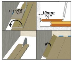
**Note:** If you are not able to angle the panels (e.g., under a door frame or low fitted radiator) you can cut away the locking edge lip of the bottom of the groove by using a wood chisel, a small block plane, or table saw. Run a bead of glue on the modified tongue and groove. Tap the panels tight together by using a hammer and push block or pull-bar. If necessary, affix it with painter's tape until the glue is dry.
