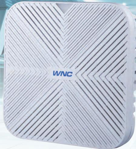
WNC's R1220 series radio unit (RU) is designed to provide 5G NR Sub-6 GHz indoor coverage and optimal 5G network access at throughput speeds of over 1 Gbps to satisfy the needs of enterprise, industrial, and commercial venues. The R1220 flexible vRAN solution reduces costs and increases connection speeds via split 7.2x fronthaul network implementation. The RU can be mounted on walls, poles or ceilings, and utilizes internal/external 4T4R antennas to boost coverage and throughput.
