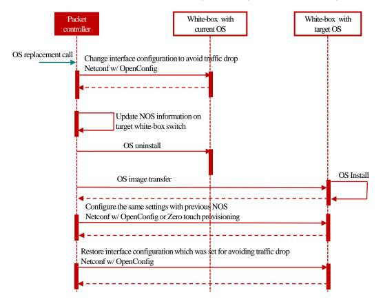
Figure 6. Workflow for automatic NOS replacement procedure
