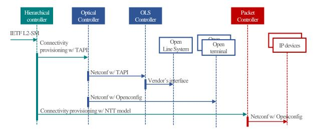
Figure 4. End-to-end provisioning workflow
