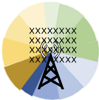
Fig. 5: A site with three cells, each cell being defined by four SSB beams, view from top
